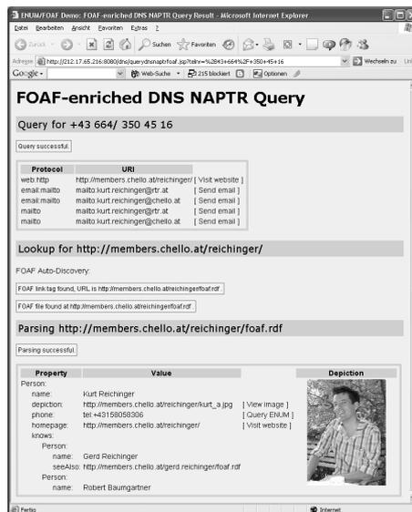
Fig. 3. Application utilising PHOAF for presentation of additional information on a contacted person or company
