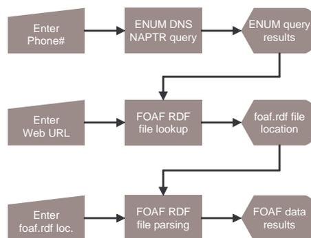
**Fig. 1.** Flowchart of JAVA prototype operations
