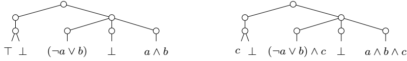
Figure 2. Tree representation of example NSF N and N[B/B \wedge c] applied to N (each BDD B is replaced with B \wedge c ).
