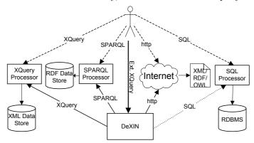
Fig. 2. Architectural overview of DeXIN framework
