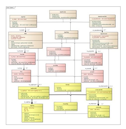
Fig. 6. The class diagram with a more complex mapping corresponding to Fig. 5  $\,$
