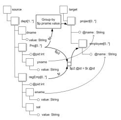
Fig. 9. A Clip mapping with a join and grouping (adapted from [13, Fig. 7])
