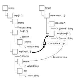
Fig. 1. A simple Clip mapping (adapted from [13, Fig. 3])
