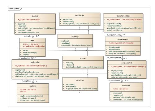
Fig. 4. The class diagram with context propagation corresponding to Fig. 3
