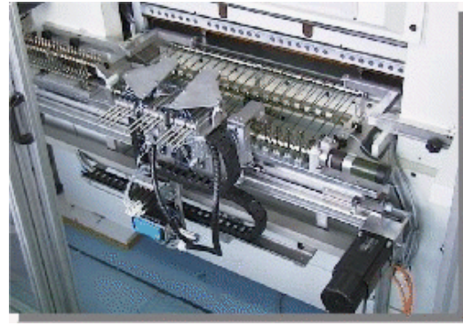
Figure 5. Transport/grip/machine feed combination in a manufacturing plant
