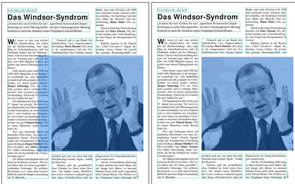
Figure 4: Page display without clipping (left) and with clipping (right) of an image
