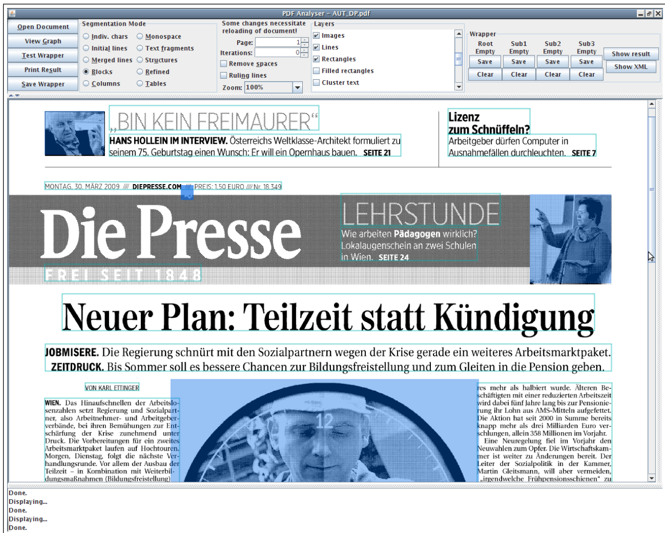
Figure 5: An example of the GUI, based on XMillum , showing the results of our segmentation algorithm overlaid on a bitmap rendition of the page
