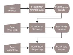
Fig. 1. Flowchart of JAVA prototype operations
